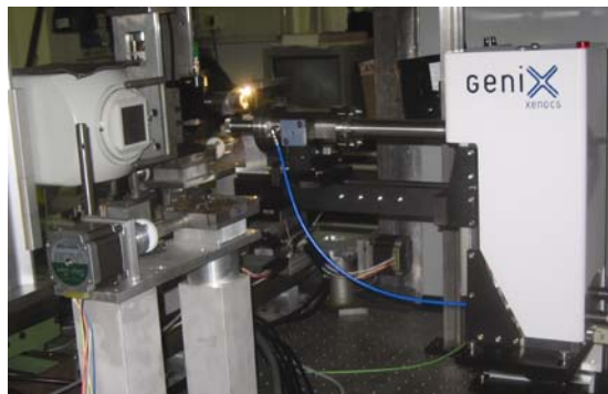
Fig. 7 : GeniX Mo Small Spot on a high pressure set up
