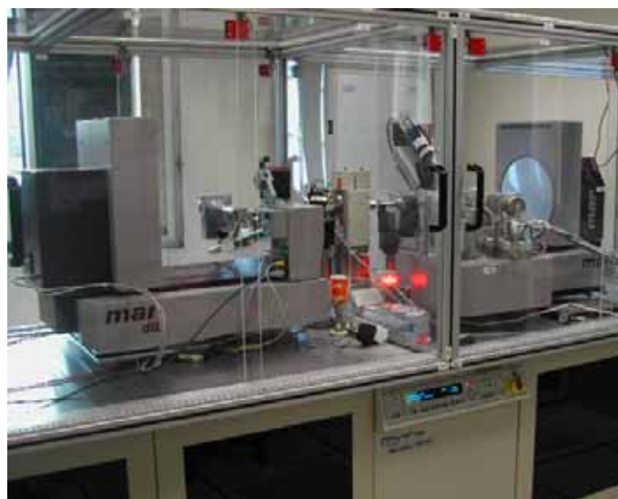
Fig. 1: Installation at Sanofi Aventis in Vitry, France with a Rigaku Micro-max 007HF Cu rotating anode generator, a MAR345 image plate detector and a FOX2D CU 25_25P optic.
