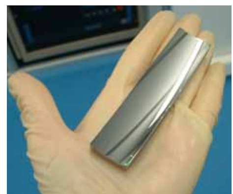
Fig. 2: Photo of a 2D aspherical analyzer (90x20mm 2 ) with a graded multilayer coating.
