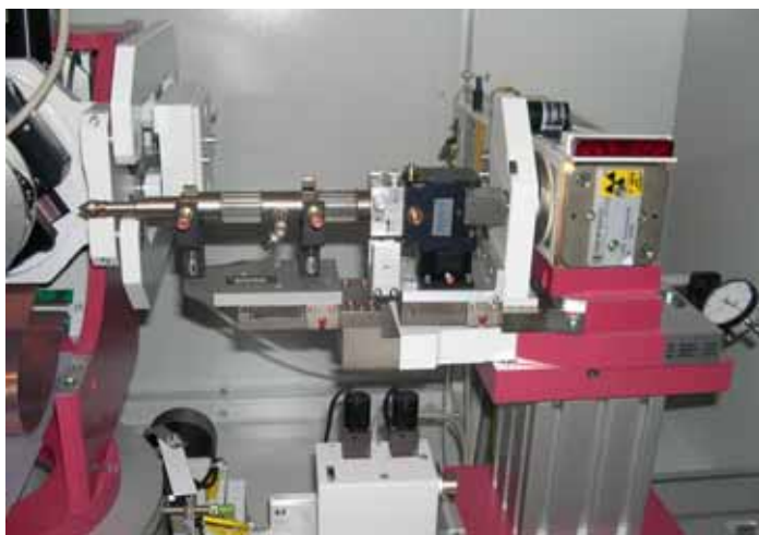
Fig. 2: Sealed tube in point focus geometry on a General Electrics IT Seifert diffractometer equipped with a FOX2D CU 12_INF mirror and an evacuated telescopic collimation system.
