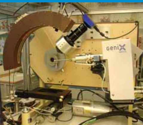
Fig. 1 : The GeniX Cu High Flux X-ray source installed at the Mineralogy Dept. of the Natural History Museum in London.
