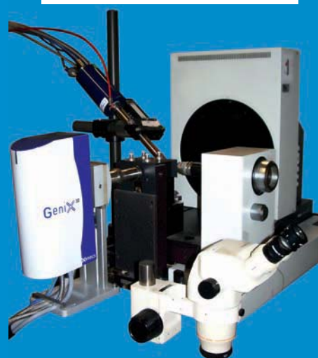
Fig.1 : The GeniX 3D Cu High Flux beam delivery system installed at the EMBL Grenoble outstation.
