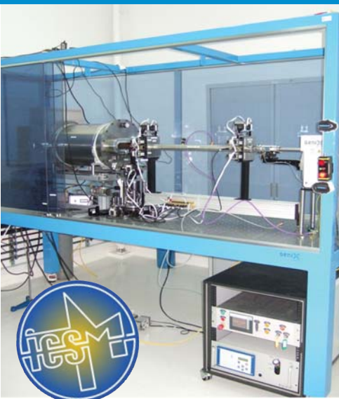
Fig. 1 : GeniX Mo Low Divergence beam delivery system installed at ICSM CEA Marcoule, France.
